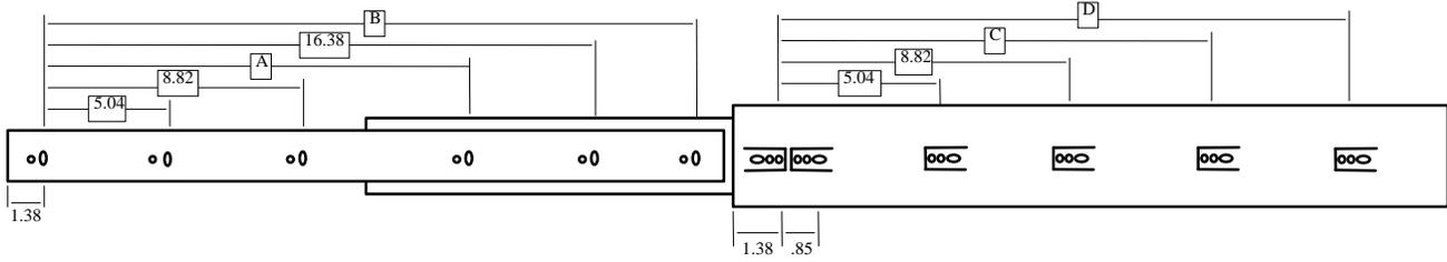
These 3-section ball bearing steel slides have full extension with quick disconnect function. They will fit into 1RU space, and can handle a full load rating of 100 lbs. per pair. A set of 4 mounting brackets and screws (16 of the 8-32 thread) are included. Standard finish is electro zinc plated. Other travel lengths and finish also available.
